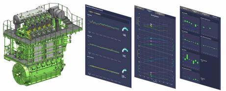
Various companies are providing platform services that automatically transmit measured data from ship to shore, and these services are increasingly being applied to new vessels. By connecting to each platform services of these companies, HiZAS is provided as web applications with various functions at minimal cost and without installing additional equipment on vessel.
